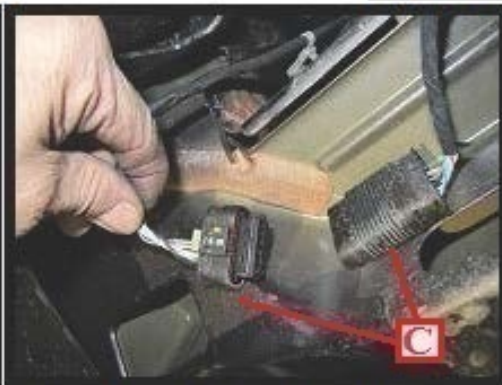
Pull out on white tab (D) in the direction of the red arrow shown in Fig. 46 to release connection lock then pull apart sensor connection (C) as shown in Fig. 79.
