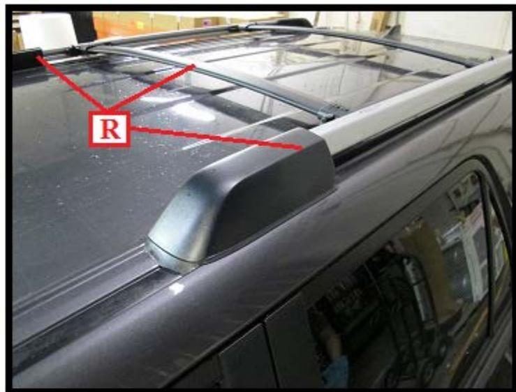
The original roof top rails (R) as shown in Fig. 1 must be removed prior to Gobi rack installation.
