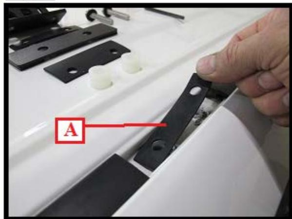
Place black seal (A) over and around each white straw tube as shown in Fig. 5 above.
