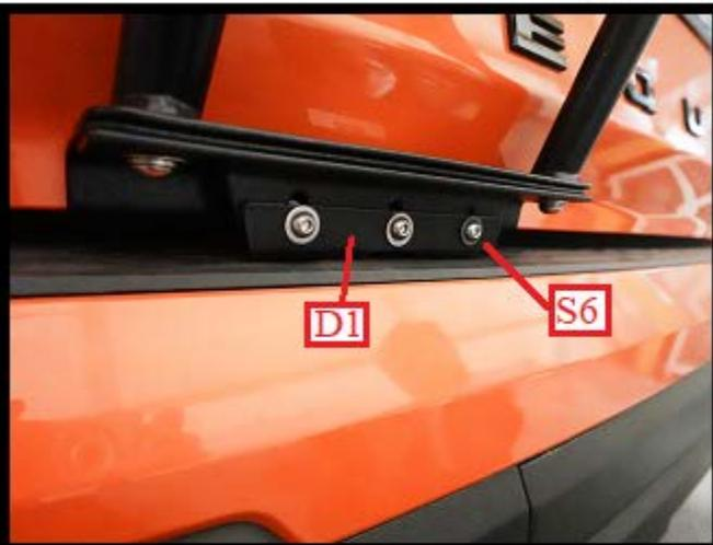
As shown in Fig. 31, using a 7/16" box end wrench and 5/32" Allen wrench, loosen and adjust the lower support plate (D1), up as high as possible (shown by red arrows) then slightly tighten the two outside screws (S6) so that they prevent plate (D1) from moving. The plate needs to be movable by hand but not fully loose. After the adjustment has been made close the door fully as shown in Fig. 32.
