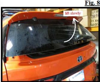
As shown in Fig. 7, after the hanger plate (C) has been temporarily installed. Check that hanger plate hook (H) clears the body (BD) of the vehicle by lifting the rear window batch slowly as shown in Fig. 8
