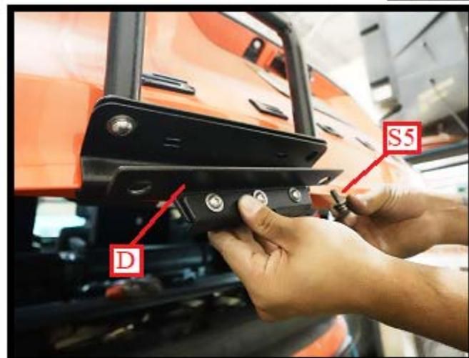
As shown in Fig. 27, tighten both screws (RC) in until you have approximately 3/16" of screw left outside jam nut (J). Then fully tighten jam nut (J) using a 3/8" box end wrench. As shown in Fig. 28, leave rear door open half way then remove one screw (S5) and install lower ladder support (D) located in your hardware kit, as shown in Fig. 29.
