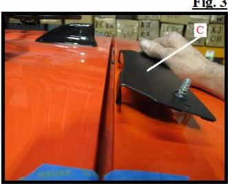
As shown in Fig. 2 and Fig. 3, clean the area of the rear spoiler with denatured alcohol where hanger plate (C) will be mounted. As shown in Fig. 3, remove hanger plate (C) from your hardware kit.
