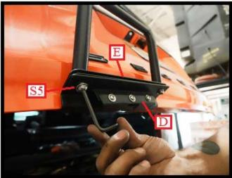
As shown in Fig. 29 and Fig. 30, remove the second screw (S5) and fully install support plate (D) shown in Fig. 30. Adjust support (D) evenly with outer edge (E) of ladder then fully tighten both screws (S5).
