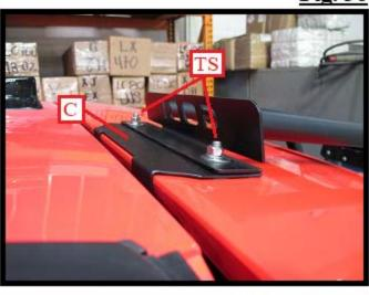
(TS) and tighten down both screws using a 1/2" box end wrench. (Do not over tighten as threaded stud can be broken). Remove all tape markers.
