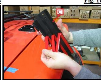
As shown in Fig. 15, remove ladder (A). As shown in Fig. 16, remove hanger plate (C) then peel off the protective double back tape covers and re-install hanger plate back in place as shown in Fig. 4 and Fig. 5.
