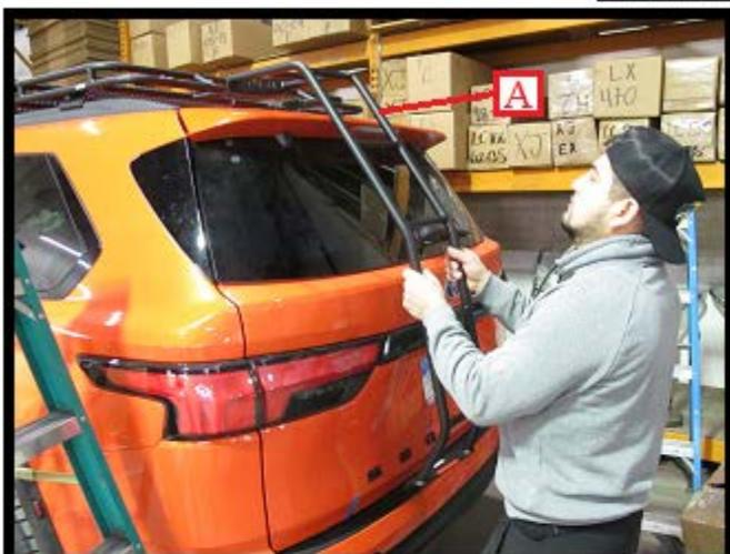
As shown in Fig. 19, make certain both 5/16-18 x 1" button head screws, lock washers and flat washers (S5) have been removed from the bottom of the ladder and placed nearby as they will be needed shortly. Peel off the protective double back tape cover. As shown in Fig. 20, set ladder (A) back up onto hanger plate (C).
