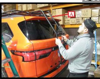
As shown in Fig. 19, make certain both 5/16-18 x 1" button head screws, lock washers and flat washers (S5) have been removed from the bottom of the ladder and placed nearby as they will be needed shortly. Peel off the protective double back tape cover. As shown in Fig. 20, set ladder (A) back up onto hanger plate (C).
