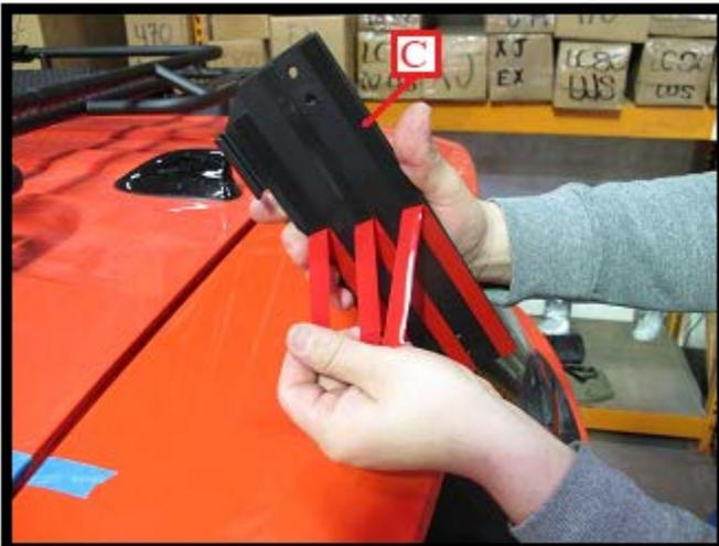
As shown in Fig. 15, remove ladder (A). As shown in Fig. 16, remove hanger plate (C) then peel off the protective double back tape covers and re-install hanger plate back in place as shown in Fig. 4 and Fig. 5.
