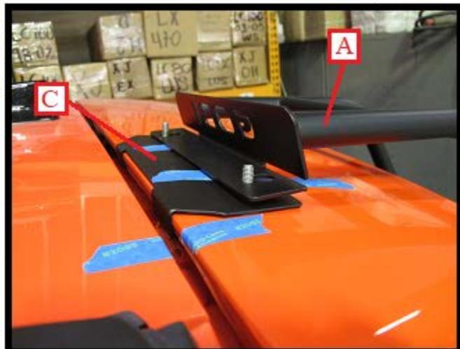
As shown in Fig. 11 and Fig. 12, set ladder (A) onto hanger plate (C) threaded studs. Allow ladder (A) to hang freely as shown in Fig. 13.
