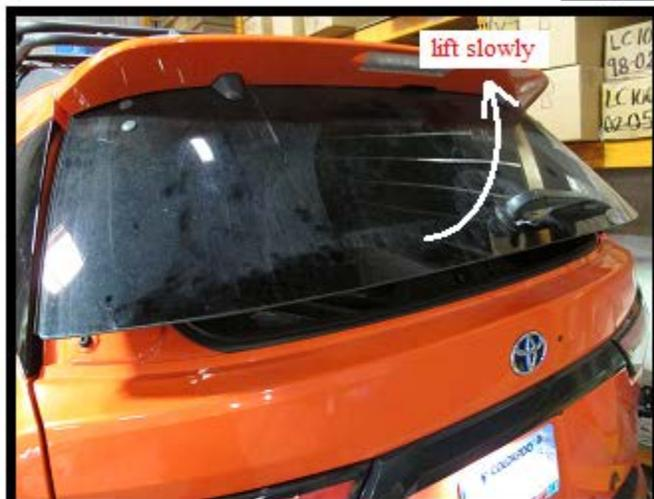
As shown in Fig. 7, after the hanger plate (C) has been temporarily installed. Check that hanger plate hook (H) clears the body (BD) of the vehicle by lifting the rear window hatch slowly as shown in Fig. 8.
