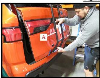
As shown in Fig. 21, pull down ladder (A) shown by white arrows with force and align the lower left-hand edge of the ladder with the masking tape marker previously set and press onto the rear door. Hold in place for 30 seconds. As shown in Fig. 22 unlock rear door and prevent the door from lifting more than a few inches. Keep the door open in place currently.
