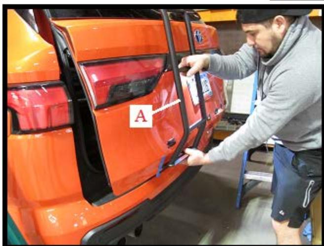
As shown in Fig. 21, pull down ladder (A) shown by white arrows with force and align the lower left-hand edge of the ladder with the masking tape marker previously set and press onto the rear door. Hold in place for 30 seconds. As shown in Fig. 22 unlock rear door and prevent the door from lifting more than a few inches. Keep the door open in place currently.
