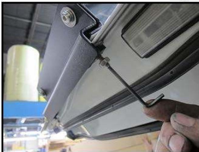
Use the short 1/8" Allen wrench located in Bag #1 of your hardware kit and tighten the two set screws located on the back of clamp plate (B) with no more than 5 to 7 lbs. torque as shown in Fig. 9. In some cases, pinch plate (2) may tilt during tightening, this will not affect the performance or strength of the ladder.
