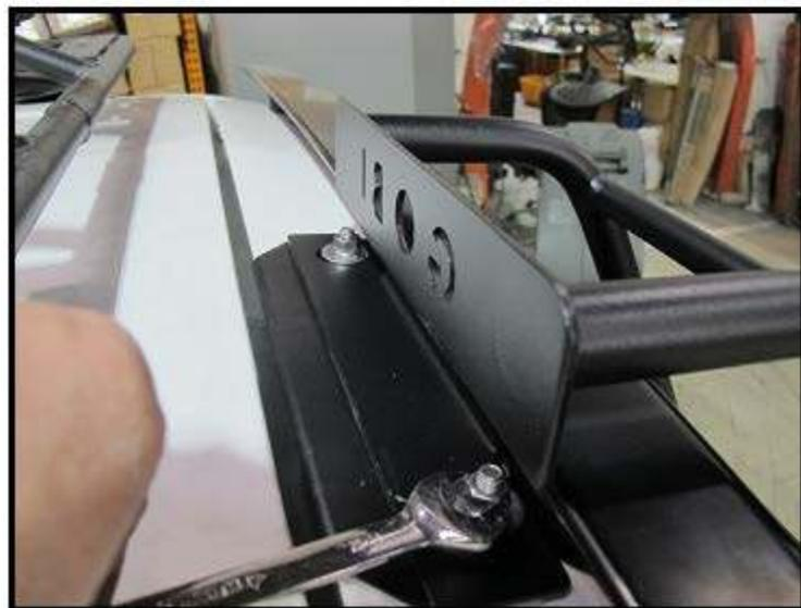
Install two neoprene washers, lock washers and nuts located in Bag #1 of your hardware kit, onto the hanger plate threaded studs as shown. Tighten down with approximately 5 lbs. of torque, do not overtighten,
