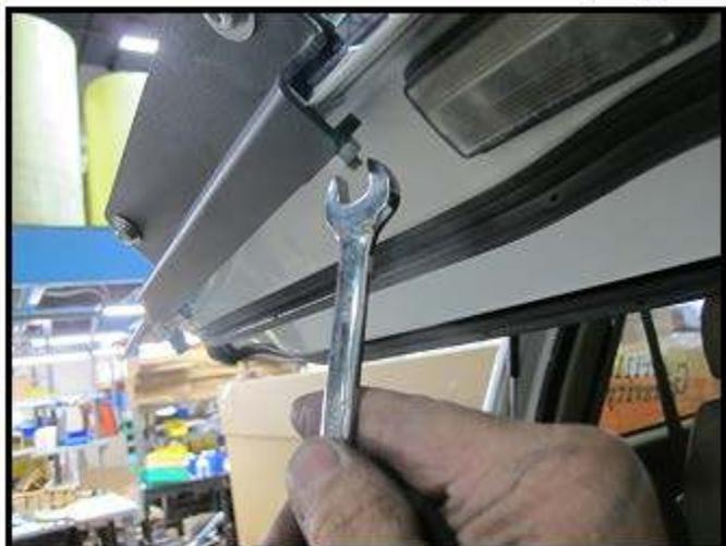
Use a 7/16" open end wrench and tighten down both nuts (B3) as shown in Fig. 10 of clamp plate (B). Use approximately 5 to 7 lbs. torque to tighten.
