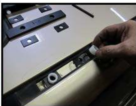
Fig. 9 Place nylon spacers over gaskets
