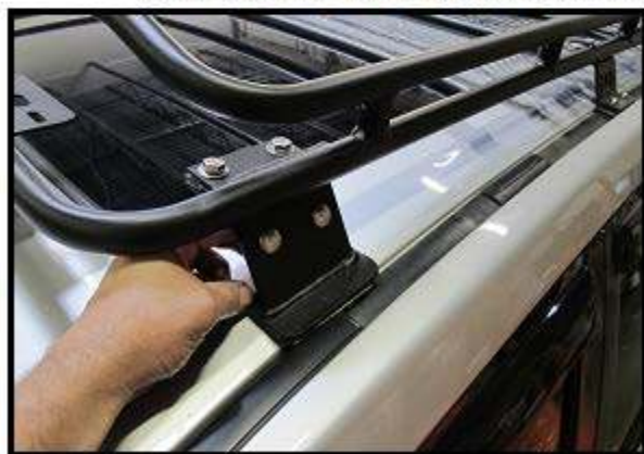
Fig. 17 Place driver side front mount bracket marked with (D) on the front driver side roof rack and install screws and rubber pad as previously completed on Fig. 16. Apply the same to the passenger side, snug down only.
