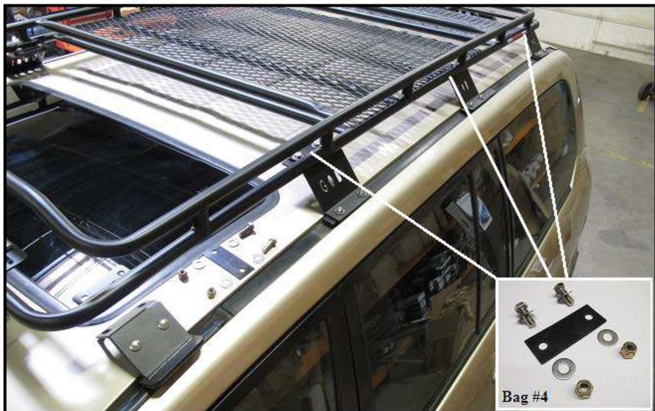
Fig. 16 Place roof rack over the 6 support brackets just previously installed and make certain to slide a black rubber pad located in Bag #4 between each weld in mounting flange/tab of the roof rack and support bracket. Install all 12 3/8-16 x 1" hex head screws, flat washers and nylock nuts and snug down only at this time.
