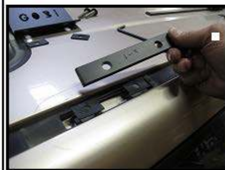
Fig. 11 Place black cover plate over gaskets
