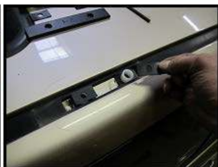
Fig. 10 Place another gasket over nylon spacers
