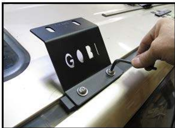
Fig. 14 Install two M8x50 screws, lock washers and water proof washers located in Bag #3 and snug down with a 5mm Allen wrench
