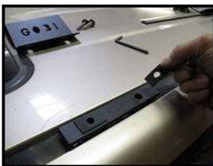
Fig. 12 Place 2 more gaskets over cover plate holes
