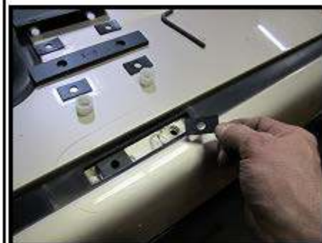
Fig. 8 Place gasket on roof top around mounting holes.
