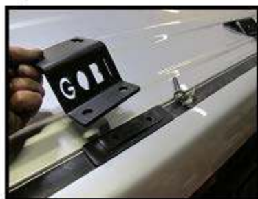
Fig. 14 Place support bracket over gasket and cover plate
