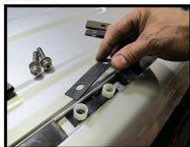
Fig. 12 Place another gasket over nylon spacers
