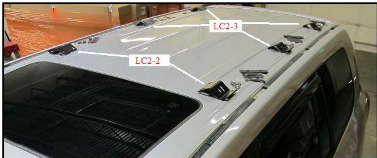
Fig. 9 Remove all dirt and debris from all mounting points and clean with denatured alcohol. Place GOBI support brackets on the roof top as follows: Support bracket (LC2-2) at the mounting point just behind the sunroof. Support brackets (LC2-3) on the remaining four mounting points as shown above.
