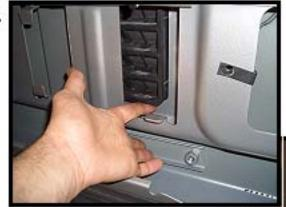
Place your index finger under the rear door vent and push up on the plastic clips both the right and left hand sides. The bottom of the vent will pop out slightly allowing you to remove the vent completly from the outer side of the door.
