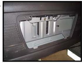
Open the H3 rear door and remove the rear door plastic access cover and all tire jack accessories with in.
