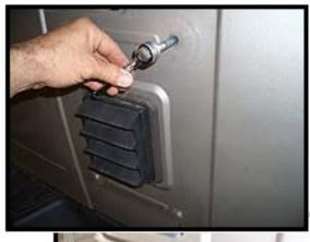
Once the rear door tire support bracket has been removed any threaded studs left in the rear door must also be removed use either a spline drive or a 1/4" hex socket drive. Remove all four (4) studs from the rear door.
