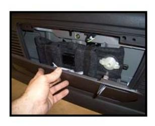
Make certain all nuts and bolts are fully tightened then re-install all jack accessories, tighten in place and finally install the rear door jack accessory plastic cover.
