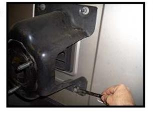
Using a 15mm box end wrench loosen all four (4) nuts of the rear tire carrier support bracket. Then continue by removing the lower 2 nuts completly. While holding the tire carrier housing with one hand remove the final two upper nuts. This will prevent the tire carrier support bracket from swinging and scratching your vehicle. If the threaded studs should come out along with each nut this is good as the threaded studs will need to be removed next.
