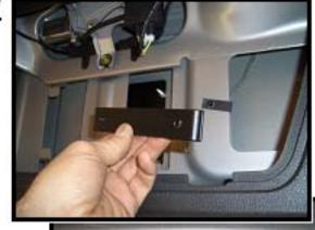
Install clamp plate with formded edges towards the back of the vent cover then over the threaded studs located on the inside of the vent cover.
