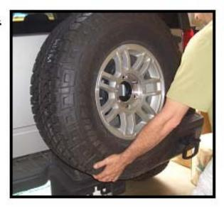
Begin by removing the rear door spare tire using the lug wrench supplied with your vehicle
